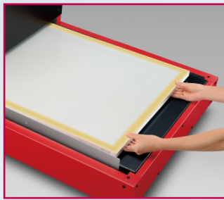
1. Set a screen stretched onto a frame
