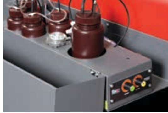
Bulk ink system with WIMS® ink circulation and filtration.
