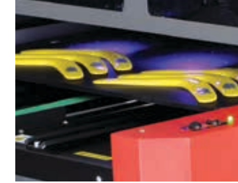
Dual water cooled LED lamps. 395Nm low heat. (iUV-350s single lamp)
